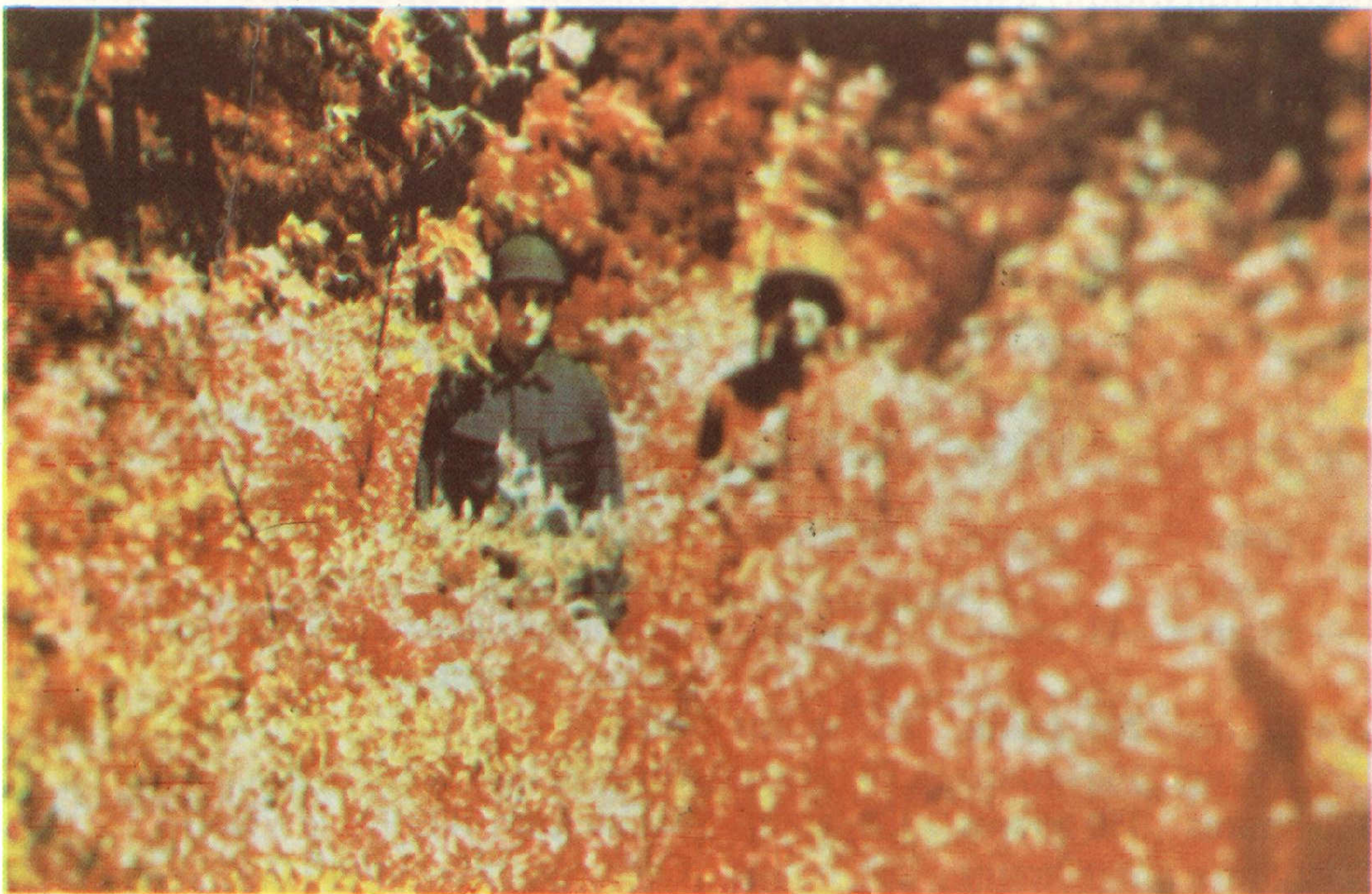
This infra-red photograph shows the effect of incorporating carbon into the camouflaged uniform material. Left: figure without carbon; Right: figure with 4% carbon.
